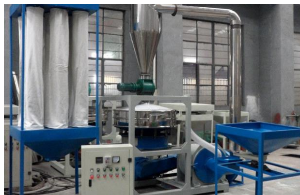
Figure 1.12: Pulverizer for UPVC Pipes and Fittings
