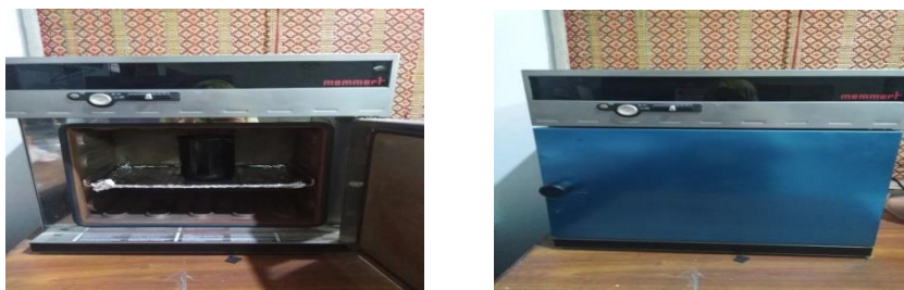
Figure 4.9 Furnace Oil Preheating in Oven
