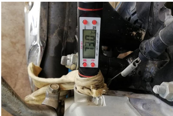
Figure 14: Oil Temperature during Operation
