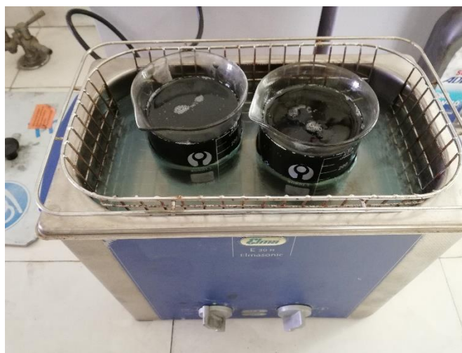
Figure 8: Water Bath Heating of Sample
