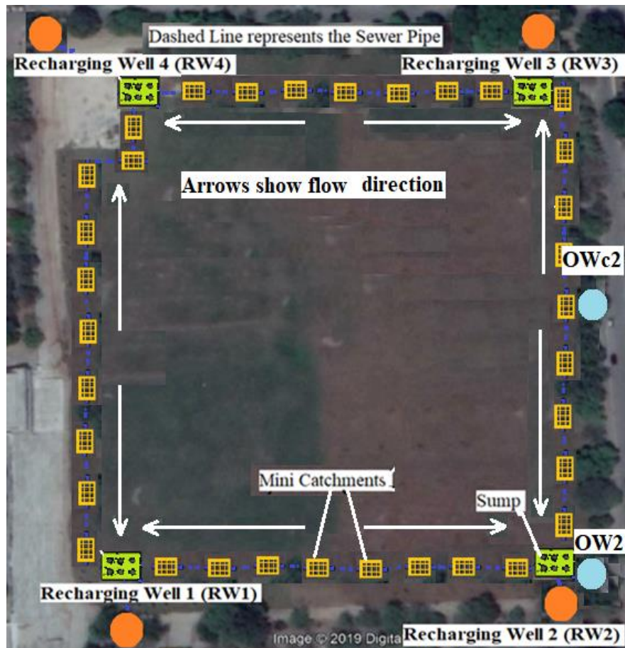
Figure 3.8 Layout of Junaid Jamshed Cricket Stadium showing installed two Piezometers
